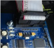
5. Route the 2 ribbon cables carefully through the opening shown and reinstall the wifi module cover and screws., The cover has a groove that needs to slide into the box edges at the ribbons.
